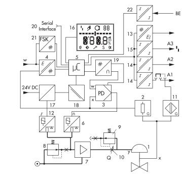
Fig. 5: Functional diagram of Type 3730-3 Positioner
